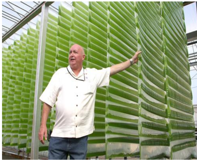
Figuur 9: Algen bioreactoren in demonstratie plant Valcent Products Ltd. Te El Paso, Texas (VS) [19]
